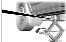
Position the head of the vehicle jack under the front sub-frame rear mounting bolts.
