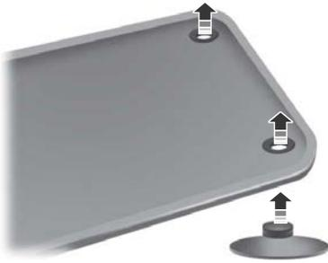
To install the floor mats, position the floor mat eyelet over the retention post and press down to lock in position.
