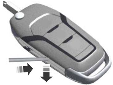
2. Insert a suitable tool, for example a screwdriver, in the position shown and gently push the clip.
