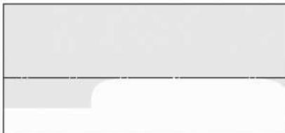
4. On the wall or screen you will observe a flat zone of high intensity light located at the top of the beam pattern. If the top edge of the flat zone of high intensity light is not on the horizontal reference line, adjust the aim of the headlamp beam.
